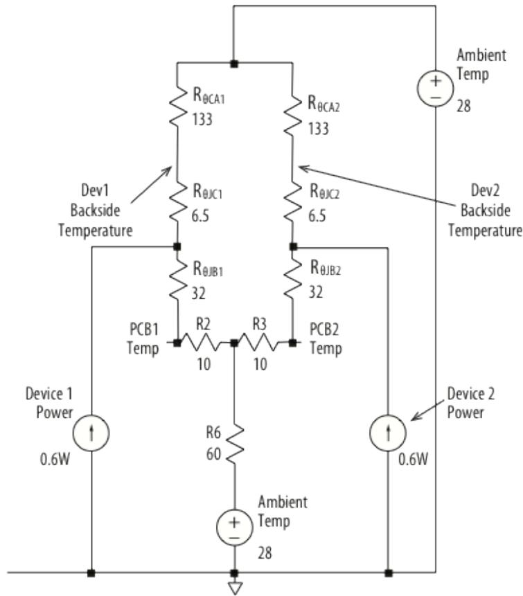
Figure 8: Electrical-equivalent circuit thermal model of the EPC9006 development board in still air without a heat sink.
