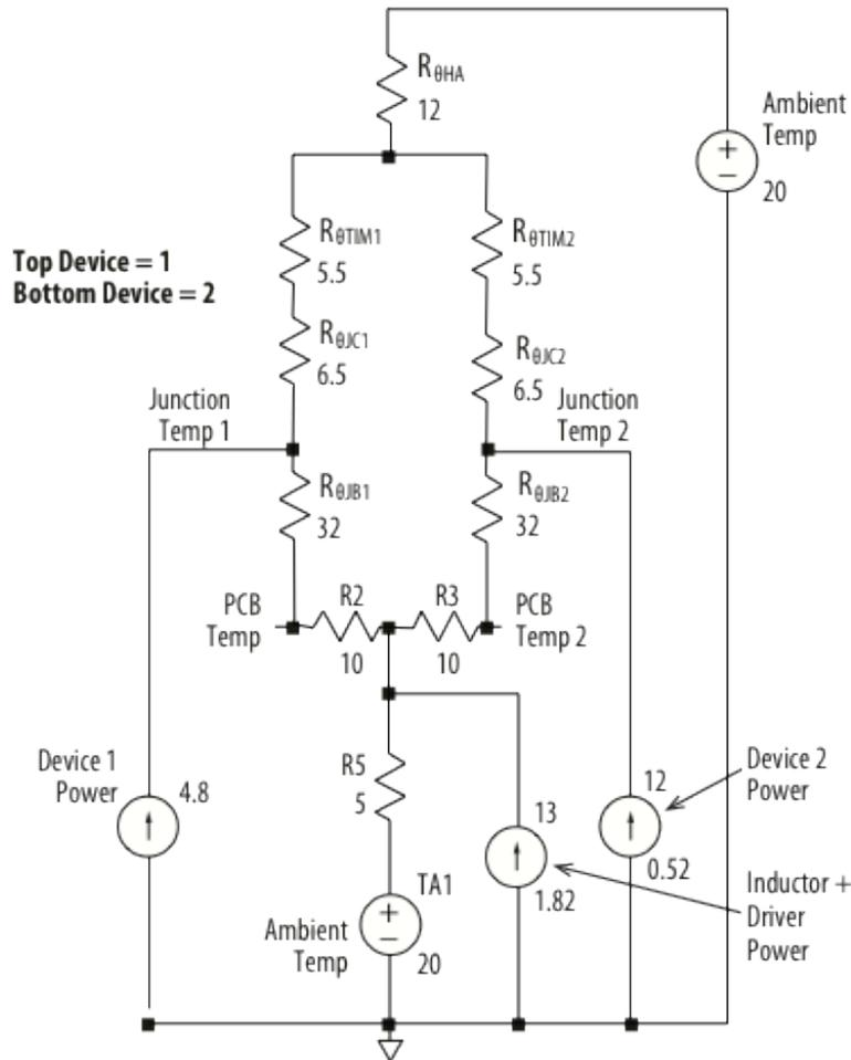
Figure 9: Electrical-equivalent circuit thermal model of the EPC9006 development board with a heat sink including power dissipation from the inductor and gate driver IC.
