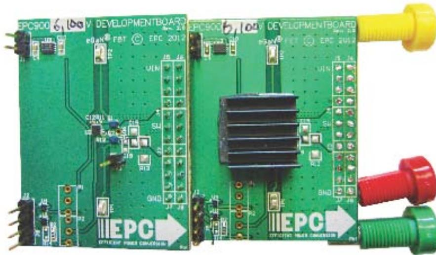
Figure 7: Standard (Left) and modified (Right) EPC9006 development boards.
