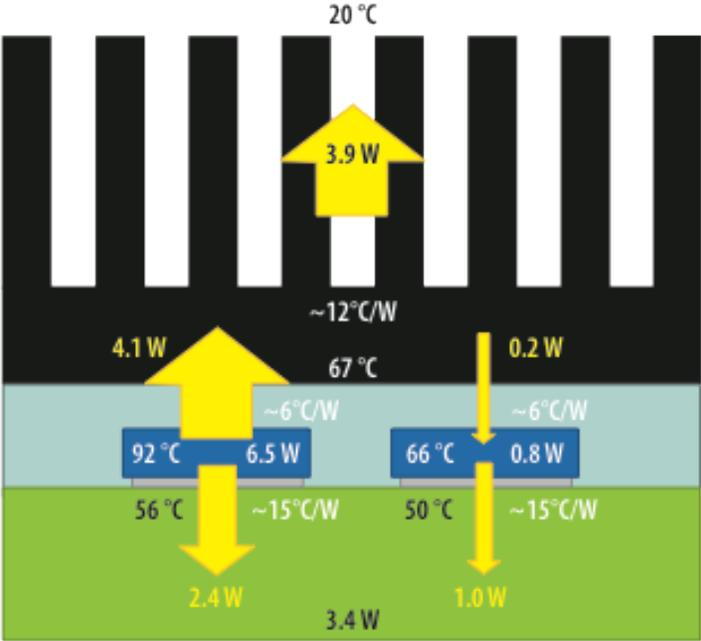
Figure 12: Estimated thermal diagram for the EPC9006 development board with a heat sink.
