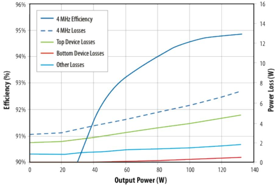
Figure 10: Efficiency and power loss of the EPC9006 demonstration board with a heat sink, operating at 4 MHz, 45 V<sub>IN</sub>, 22 V<sub>OUT</sub>.
