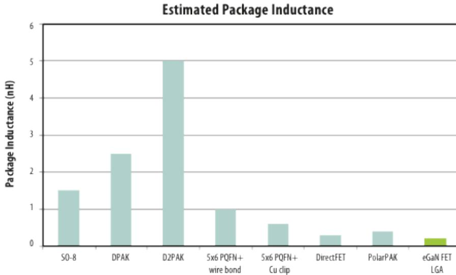
Figure 3: Estimated die free package inductance for different power packages. (eGaN FET inductance is for EPC2001, EPC2015, and EPC2010. Smaller die have higher inductance).
