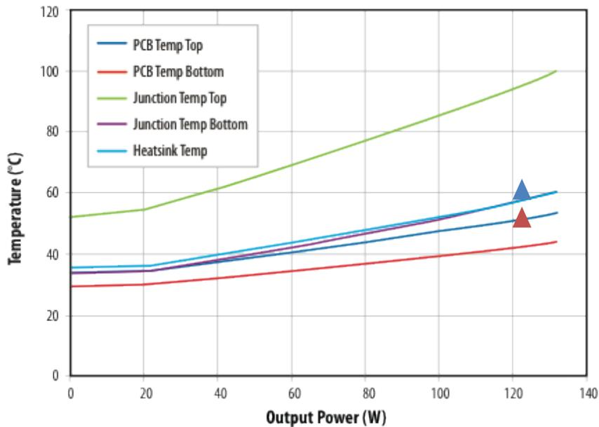
Figure 11: The temperatures of the PCB, heat sink, and device's junction with a heat sink and 200 LFM airflow. Triangles represent actual measured values.
