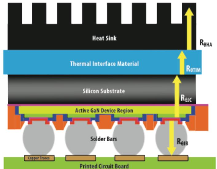
Figure 4: Not-to-scale cross-section of an eGaN FET mounted on a PCB and with a heat sink mounted on the top surface for additional cooling.
