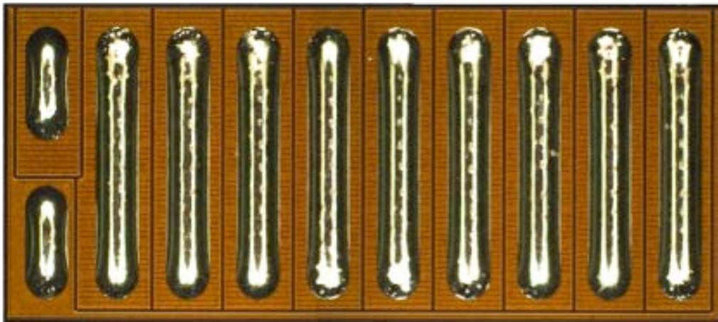
*Figure 1: The EPC2001 eGaN FET is rated at 100 V, 7 m $\Omega$  and 25 A. This LGA package has a length of 4.1 mm and a width of 1.6 mm.*
