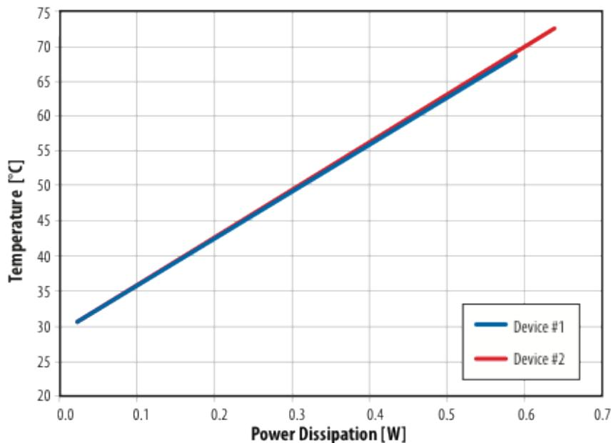
Figure 5: Without a heat sink and mounted on a standard FR4, 4-layer, 2 ounce copper PCB, the two EPC2007 eGaN FETs' junction temperatures rise to 70°C with 0.6 W of power dissipation in an ambient of 28°C.
