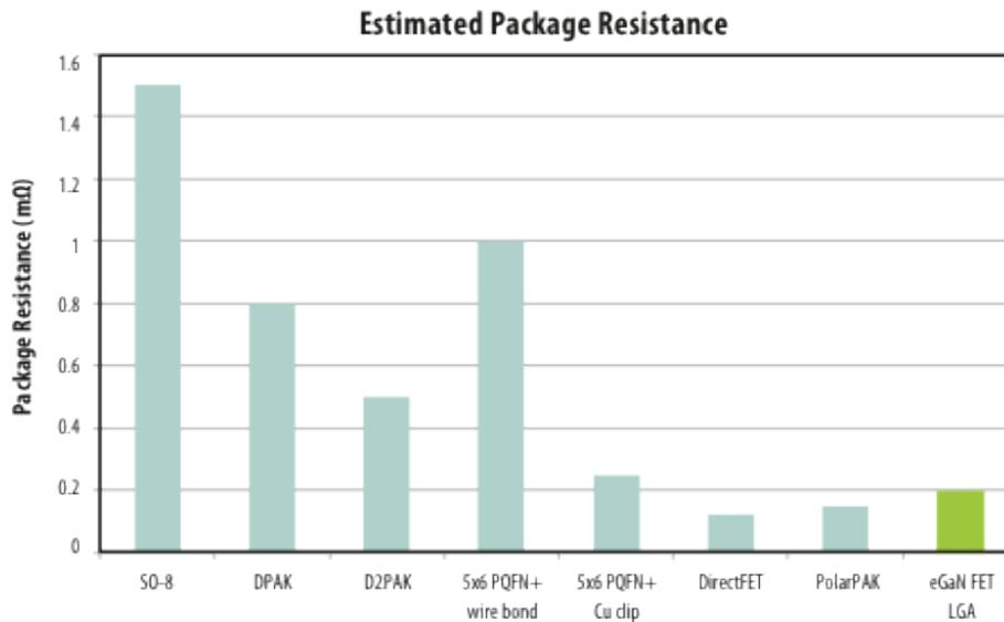
Figure 2: Estimated die free package resistance for different power packages (eGaN FET resistance is for EPC2001, EPC2015, and EPC2010. Smaller die have higher resistance).
